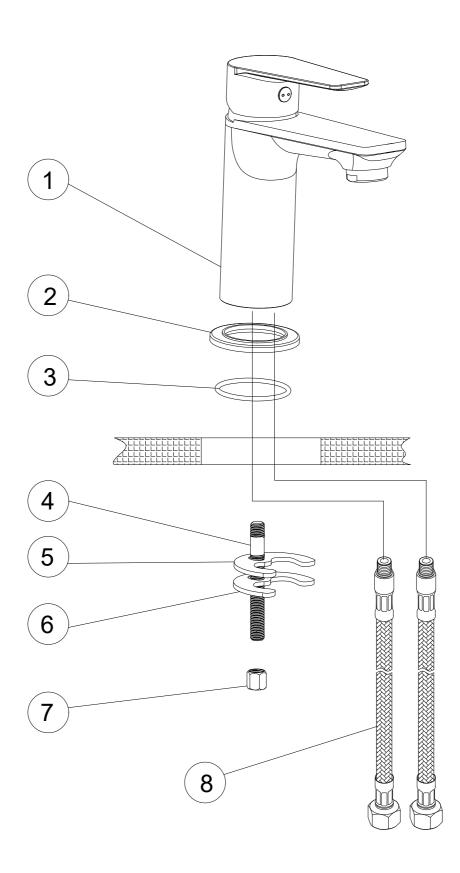
A. Secure the body of the faucet (1) by twisting the threaded rod (4). Be careful not to twist too hard. B.Place the faucet on the selected sink or board and set the base ring (2) gasket (3) between the body of the faucet and foundation. Then, set the rubber gasket (5) and metal gasket (6) onto the threaded rods (4) and tighten the nut (7).
